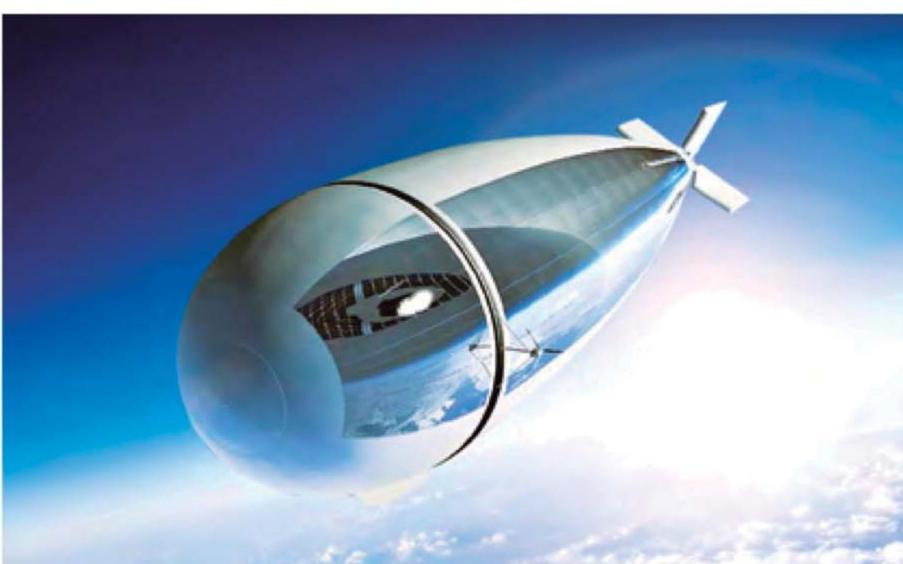
Halfway between a drone and a satellite, Stratobus is a multimission autonomous stratospheric platform. It can handle environmental missions, including marine pollution, deforestation, humanitarian aid ... © Thales Alenia Space
