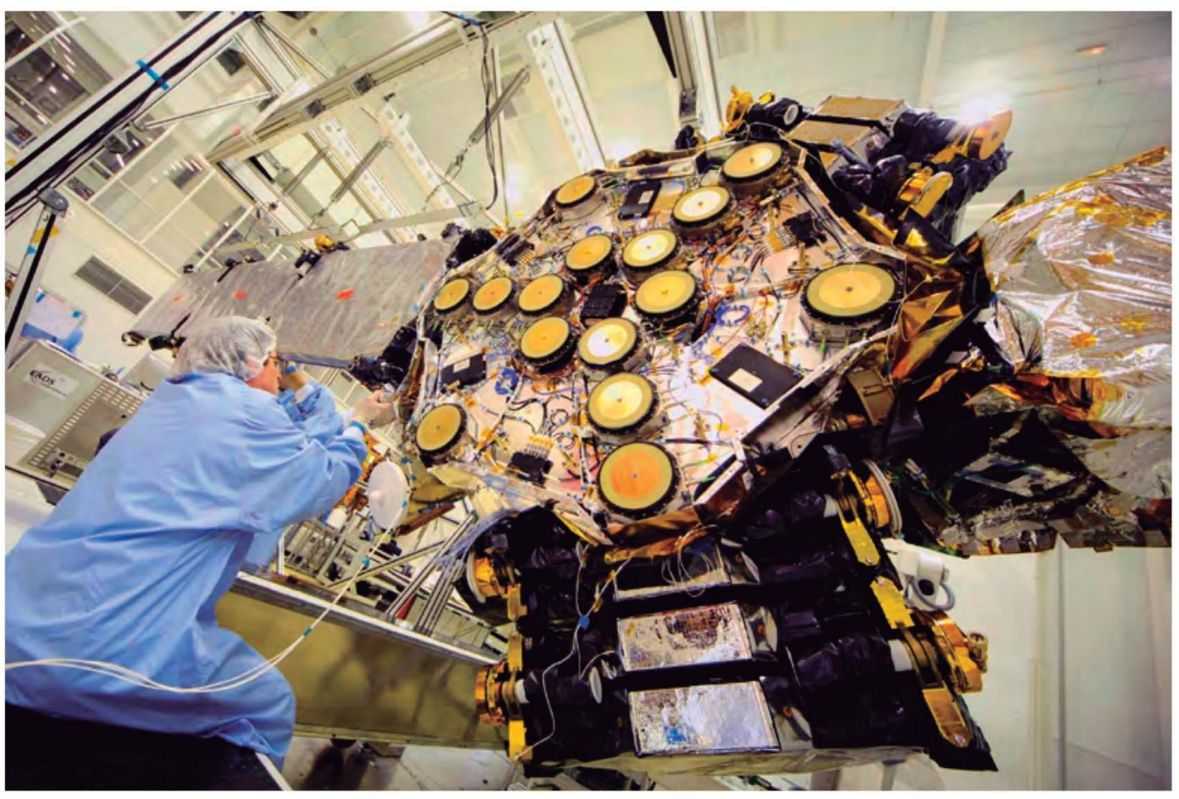
The SMOS (Soil Moisture and Ocean Salinity) ESA satellite, launched in 2009, in integration. In the foreground, the radiometer. The objective of the mission - recently extended until 2017 - is to provide maps of soil humidity and ocean salinity. © Thales Alenia Space/Yoann Obrenovitch
