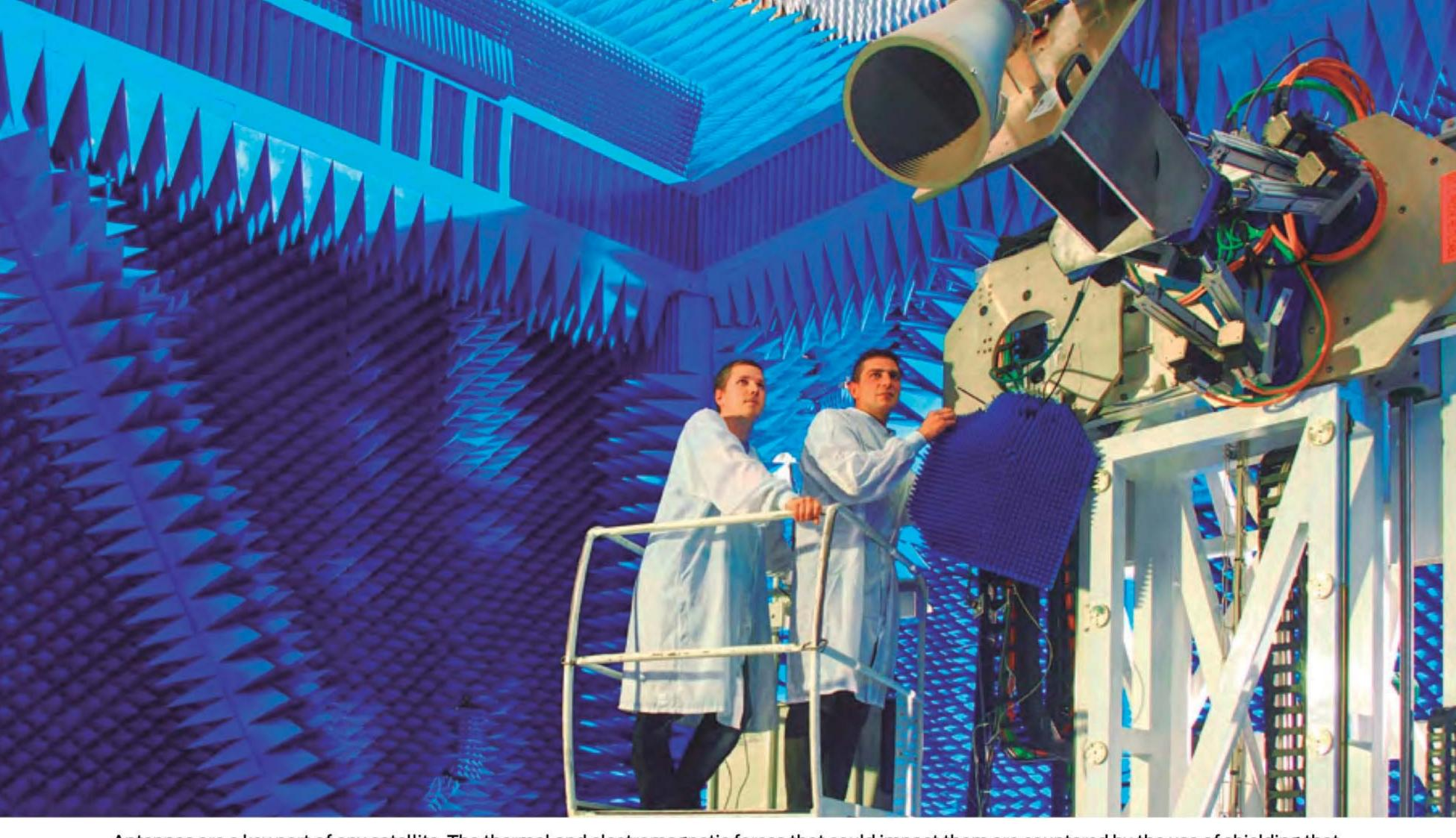
Antennas are a key part of any satellite. The thermal and electromagnetic forces that could impact them are countered by the use of shielding that ensures electromagnetic compatibility (EMC) and other arrangements. Here under test in Thales Alenia Space's clean rooms. © J.-D. Dallet/Suds-Concepts
