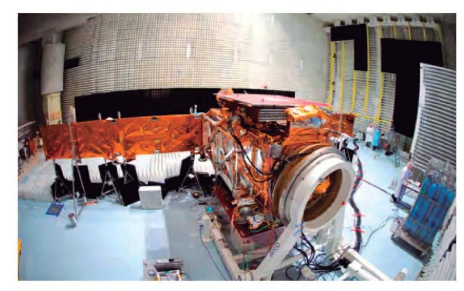
Sentinel-1A satellite in the anechoic test chamber during radio frequency tests, at Thales Alenia Space. © S. Corvaja/ESA
