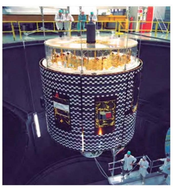
Meteosat Second Generation (MSG) testing at ESTEC (1998). © ESA
