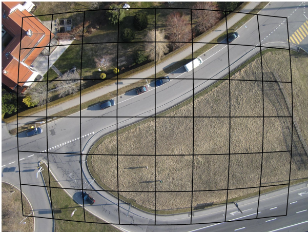
Original image: The square grid is distorted because of the lens of the camera.
